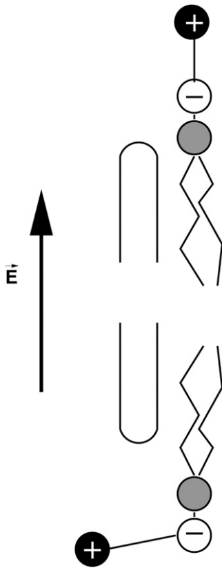
FIGURE 9 Schematic indicating the reorientation of the headgroups of the lipids close to the carbon nanotube, due to the application of the transmembrane electric field. On the side where the electric field points away from the membrane, the ammonium group of the phospholipid (black) is pushed toward the membrane and thus also over the carbon nanotube rim (indicated by an arc). On the other side, the headgroups of the lipids are stretched and the ammonium group is pulled away from the membrane. The phosphate group is indicated by a white sphere.
