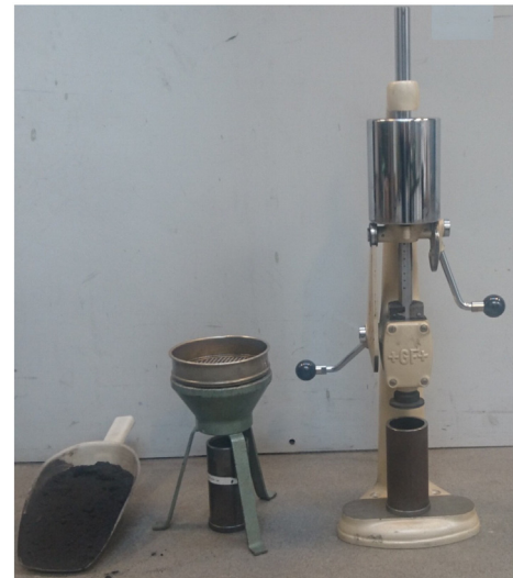
Fig. 2. Green sand (left), sieving the green sand into the cylinder (middle) and the ramming station used to determine the compactability of the sand mixture (right).
