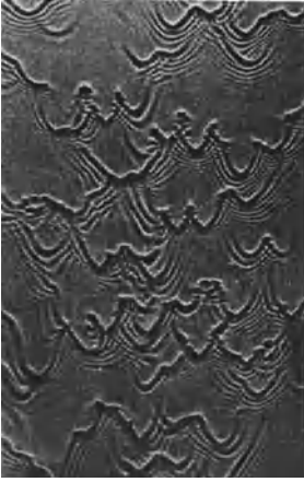
Figure 1; Waves on falling liquid film.
