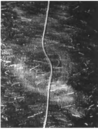
Figure 11; Hasimoto's soliton (spiral solitary wave on vortex filament).
