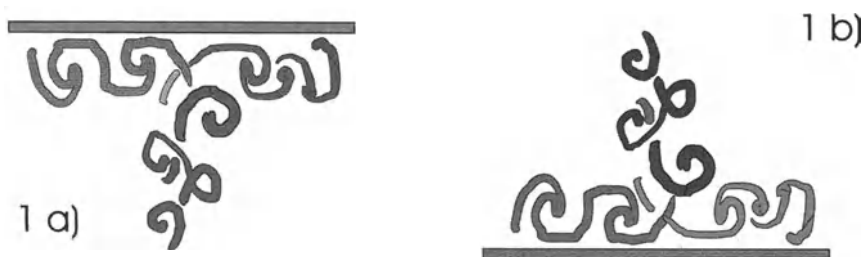
Figure 1. Density currents and thermal flows a) \rho < \rho_{umg} , b) \rho > \rho_{umg}
