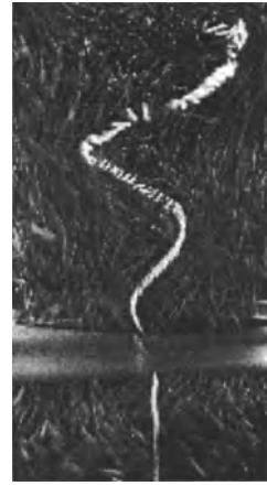
Figure 12; Vortex breakdown of spiral type.
