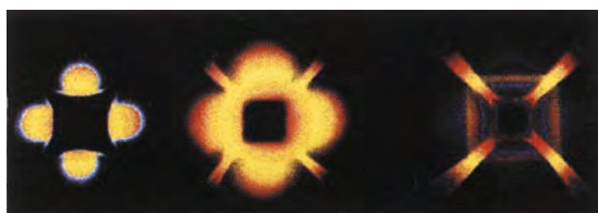
Figure 18; Formation of horseshoe structures in liquid layer with local heat source, t^{\circ}\text{C} .
