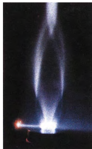
Figure 19; Supersonic ring jet (visualization with an electronic beam).
