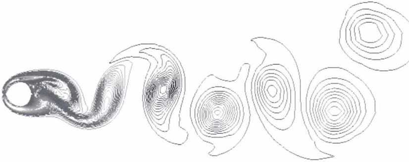
Figure 5.6. Vorticity contours of vortex shedding behind a circular cylinder at Re = 200 , using a variable blob vortex method.
