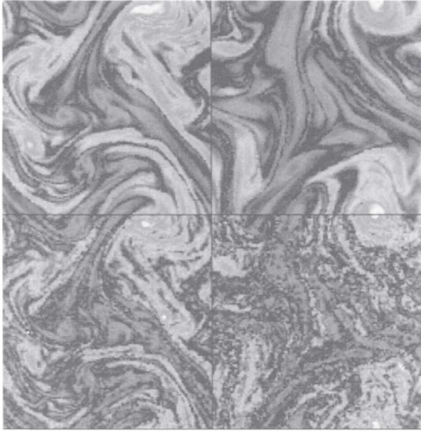
Figure 5.10. Successive stages, from left to right, in the evolution of a random vorticity field in an inviscid calculation (bottom pictures) and with the LES model of Eq. (5.6.7) (top pictures).
