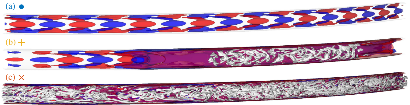
FIG. 3. Snapshots of the flow for \delta = 0.022 , \text{Re} = 5050 along the three trajectories in Fig. 4. (a) corresponds to the (blue) traveling wave, (b) to the intermediate (orange) trajectory that returns to the traveling wave, while (c) is along the (red) trajectory that converges to sustained turbulence.
