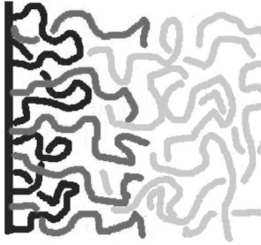
Fig. 4. Schematic representation of the molecular structure of a BPA-PC melt adjacent to a Ni wall, showing double-ended adsorbed, single-ended adsorbed, and non-adsorbed chains. (See Plate 13 on Page 275)
