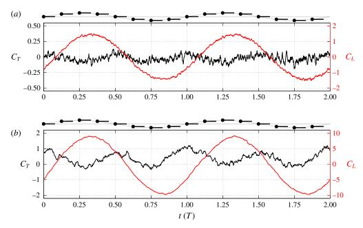
FIGURE 7. Instantaneous thrust (black) and lift (red) coefficients for the heaving foil in simulation. (a) von Kármán wake with average drag ( $St_D = 0.11$  and  $A_D = 1.20$ ) and (b) inverted von Kármán wake with average thrust ( $St_D = 0.22$  and  $A_D = 1.80$ ).
