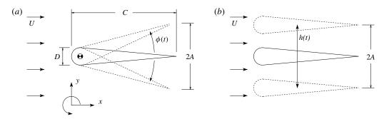
FIGURE 1. Geometry and kinematics of the foil. (a) Pure pitching and (b) pure heaving.
