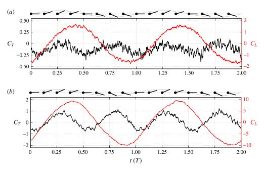
FIGURE 4. Instantaneous thrust (black) and lift (red) coefficients for the pitching foil in the simulation. (a) von Kármán wake (cf. figure 2c) with average drag ( $St_D = 0.12$  and  $A_D = 1.14$ ) and (b) inverted von Kármán wake with average thrust ( $St_D = 0.22$  and  $A_D = 1.81$ ).
